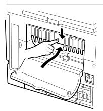
**Return the paper guide to the original position.** Raise the top edge of the paper guide and push it down to lock the paper guide in position.
