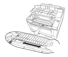
Open the upper door and remove the print unit. Be careful not to damage the green drum surface. Look for dust on the paper guide before the corona wire. Use a clean, lint free cloth to gently remove any dust from the entire surface of the paper guide.
