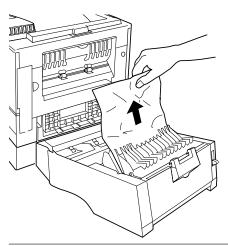
**Close the rear unit.** After removing the sheet, close the rear unit until its lock latches. Be sure to return the paper guide to the original position if it is drawn out.
