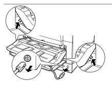
1. Disconnect the feeder cable and push the two levers at the bottom of the feeder upwards to unlock the two hooks.
