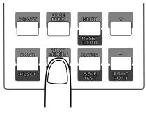
3. Set the physical paper size of the MFF. Use the MFF paper size menu to select the size of paper loaded in the MFF. See the early section in this chapter.
