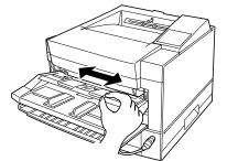
1. **Adjust the paper guides.** Position the left and right upper guides to the width of the sheet. (Lower two guides are for paper stack.)
