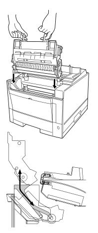
3. **Lower the print unit into the printer.** Grasp the print unit by its green handles with the green drum surface facing you.
