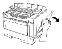
1. **Open the upper door and right side cover of the printer.** You will see a small cover on the metal plate. Remove the fastening screw and the cover. You can now see three connectors (upper two *ivory* ones for RAM cards).
