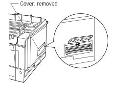
2. **Orient the RAM card.** Hold the card with the cut corner down and facing left and insert the card aslant into connector.
