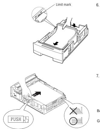
6. **Load the paper.** Place the front portion of the paper stack on the tray and slide it backwards so that the stack is placed under the two stoppers. Gather the edges of the stack together to ensure correct positioning of paper in the tray.
