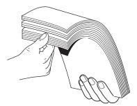
5. **Prepare a paper stack.** Prepare paper of the size indicated by the size label. Fan the paper stack both ways to prevent sheets from sticking together.
