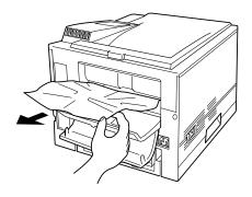
**Remove the sheet**. Pull the jammed sheet gently not so as to remain pieces of paper in the printer.
