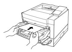
2. Place the sheet with print side face up. When the printer is ready to print, it displays the message Insert *size* to prompt you to prepare a sheet of paper. Insert the sheet until it is stopped by the feed rollers. Insufficient insertion prevents paper from being fed or causes skewed feeding.
