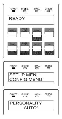
1. Enter setup mode. Press the <u>READY</u> button to put the printer offline (the ONLINE indicator turns off). Then, press the <u>MENU</u> button briefly six times.
