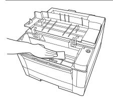
5. **Clean the inside of the printer.** Look for spilled toner inside the printer. Clean away any toner with a damp cloth.
