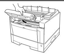
both projecting guides of the toner cartridge into the grooves of the print unit.
