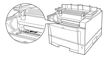
Remove the print unit and store it in a dark, level, steady place. Be careful not to damage the green drum surface. Using the tool as shown in this figure, clean the corona wire. Fit the positioning cut onto the wire housing frame and gently move the tool left and right two or three times along the length of the wire to remove any dirt or other substance. Be careful not to break or otherwise damage the wire.
