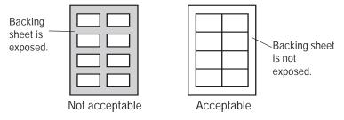
• Test-print labels before using them. If jamming problems occur and continue, try a different type of label.
