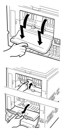
4c. Open the rear stacker at the back of the printer.
