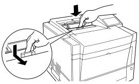
9. **Lock the cleaner.** Push down the top of the handle and pull it towards you to lock the cleaner.
