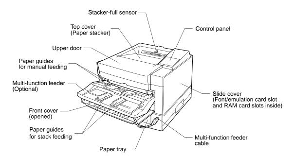
Figure 1–1 Front and right side view
