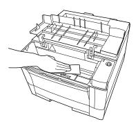
Open the upper door and remove the print unit. Be careful not to damage the green drum surface. Look for spilled toner on the inside of the printer. Use a damp cloth to remove any toner stains.
