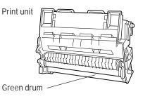
To avoid spilling toner, be sure to keep the print unit upright and keep the toner cartridge mounted on the print unit.
