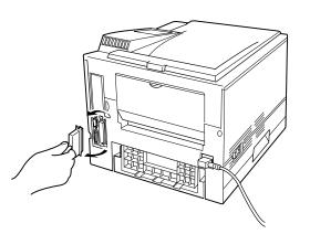
To make the connection, plug the cable connector into the parallel interface port on the back of the printer. Secure the connector with the wire clips. Plug the other connector into your computer's parallel port. Consult your computer documentation if you need help.
