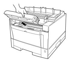
3. Unlock and remove the old toner cartridge. Pull the top of the toner cartridge toward you to swing the cartridge from the upright position to the removable position. Gently remove the cartridge. If necessary, clean toner around the toner hopper entry of the print unit.
