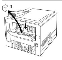
10. Remove the protective material from the rear stacker. Open the rear stacker and remove restraint cushion q. Make sure the paper guide is pushed down in the locked position. Close the rear stacker.
