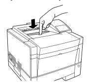
1. **Open the cover.** Push the engraved portion on the stacker to unlock the cover.
