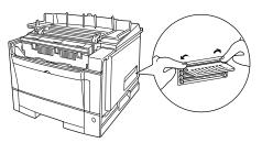
To remove an unsealed RAM card push out the retaining clips. When, the card slants outwards pull the card to remove.
